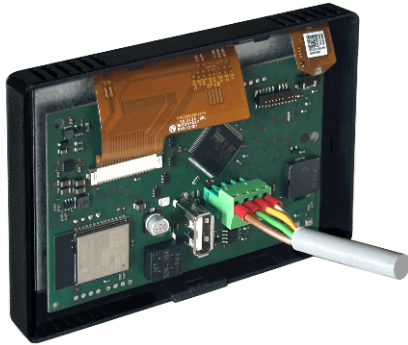
Clamp with inserted cable for connection to the display
